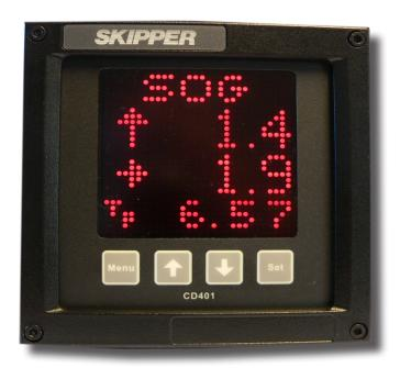
The SKIPPER CD401CU is a Control unit for the DL1 Doppler speed log, with interfaces to the DL1 JB70D1 unit via LAN or NMEA cabling. THe unit gives full control of the DL1 system, and has a web page for simple configuration.
